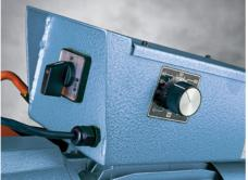
**Variable Speed Control** (Not Available on NF or 275 series) Recommended for cutting multiple shapes, sizes, and thicknesses. RPM can be fine-tuned to achieve optimum
