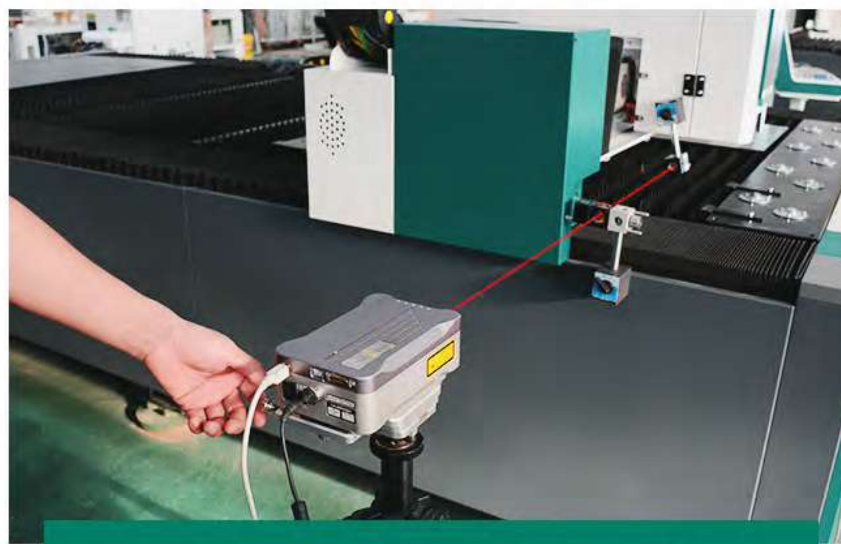
Positioning Accuracy Inspection
