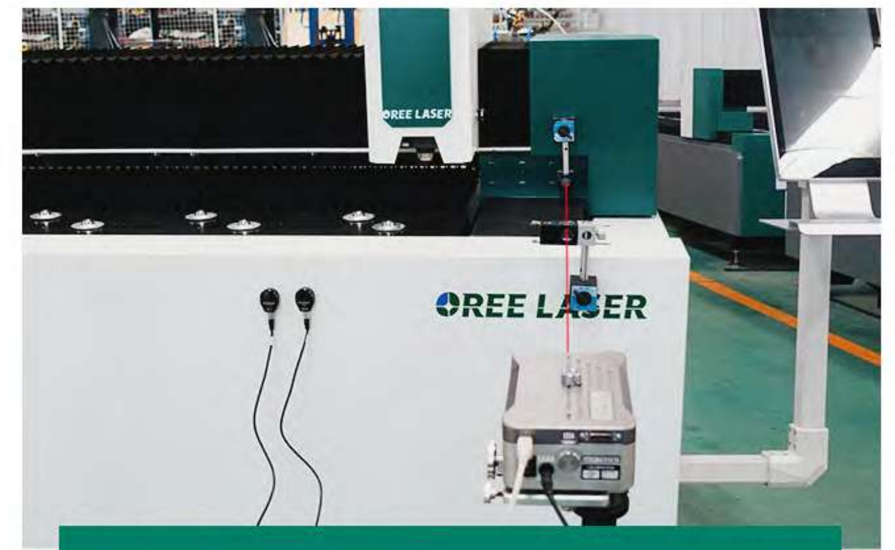
Positioning Accuracy Inspection
