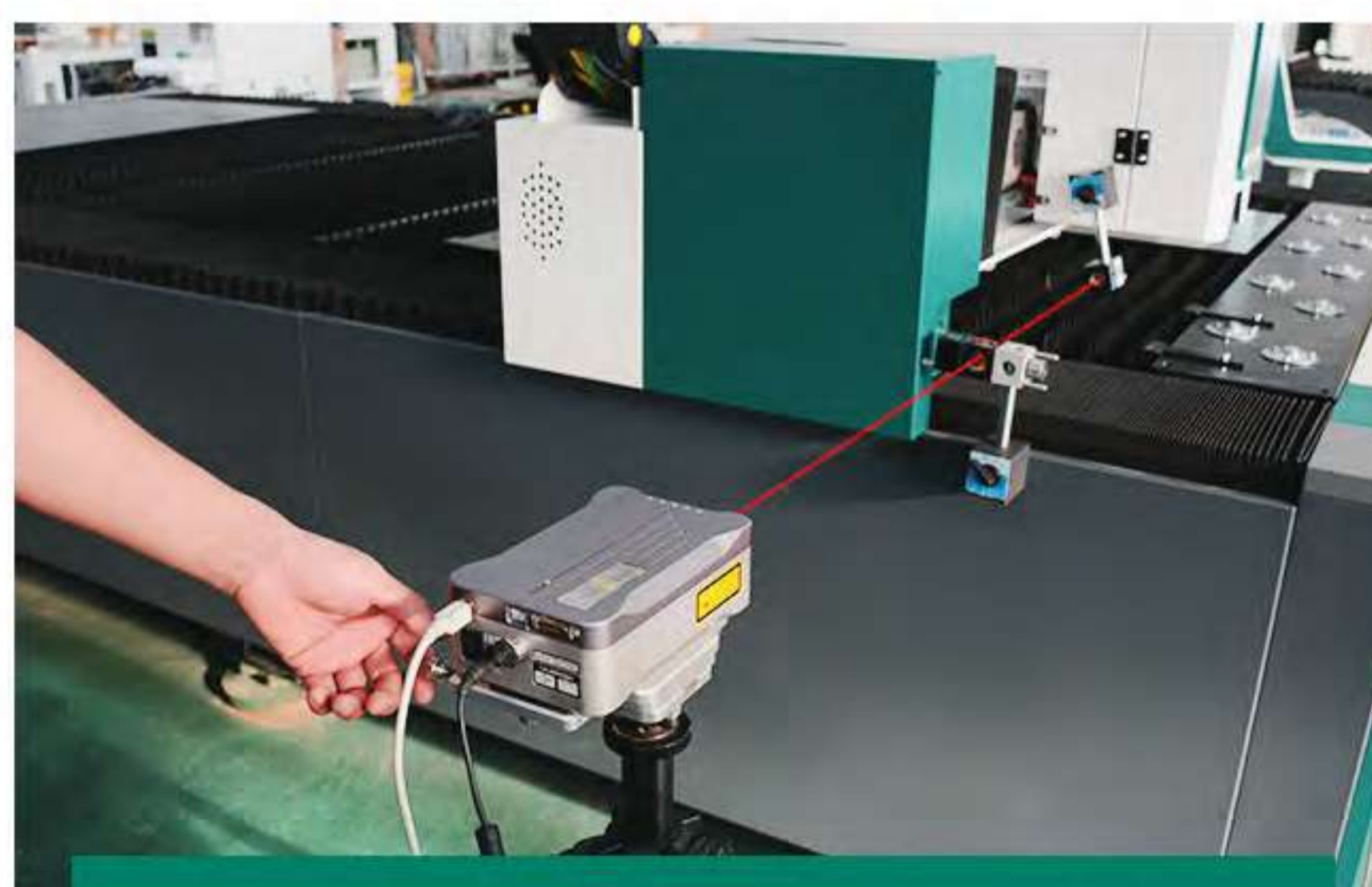
Positioning Accuracy Inspection
