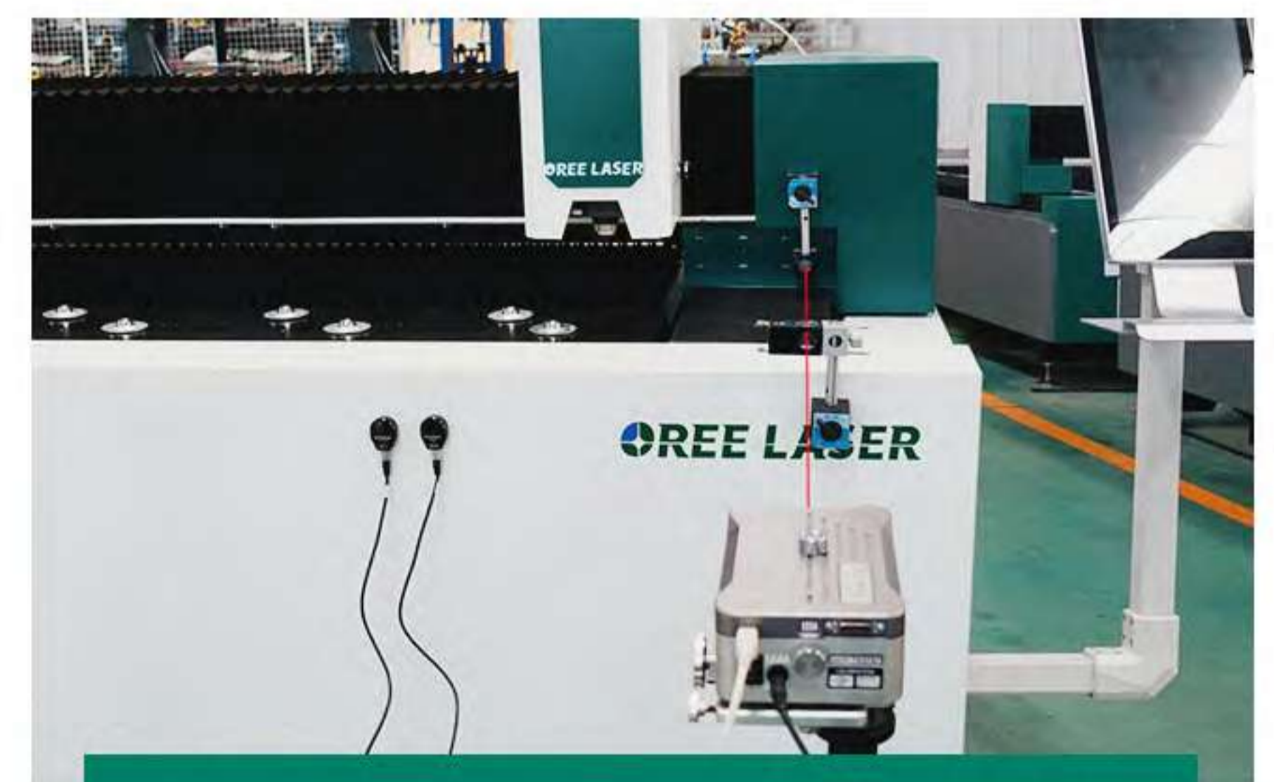
Positioning Accuracy Inspection
