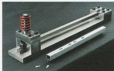
Add a Multicyl to a Mandrel Die for long components
