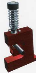
Pierce round or shaped tubes with dimpled holes through one or both sides
