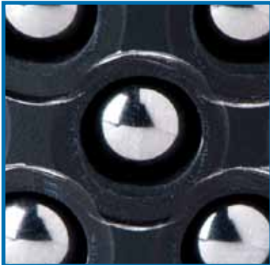
Figure 3: Stake Stress – Two-Point
